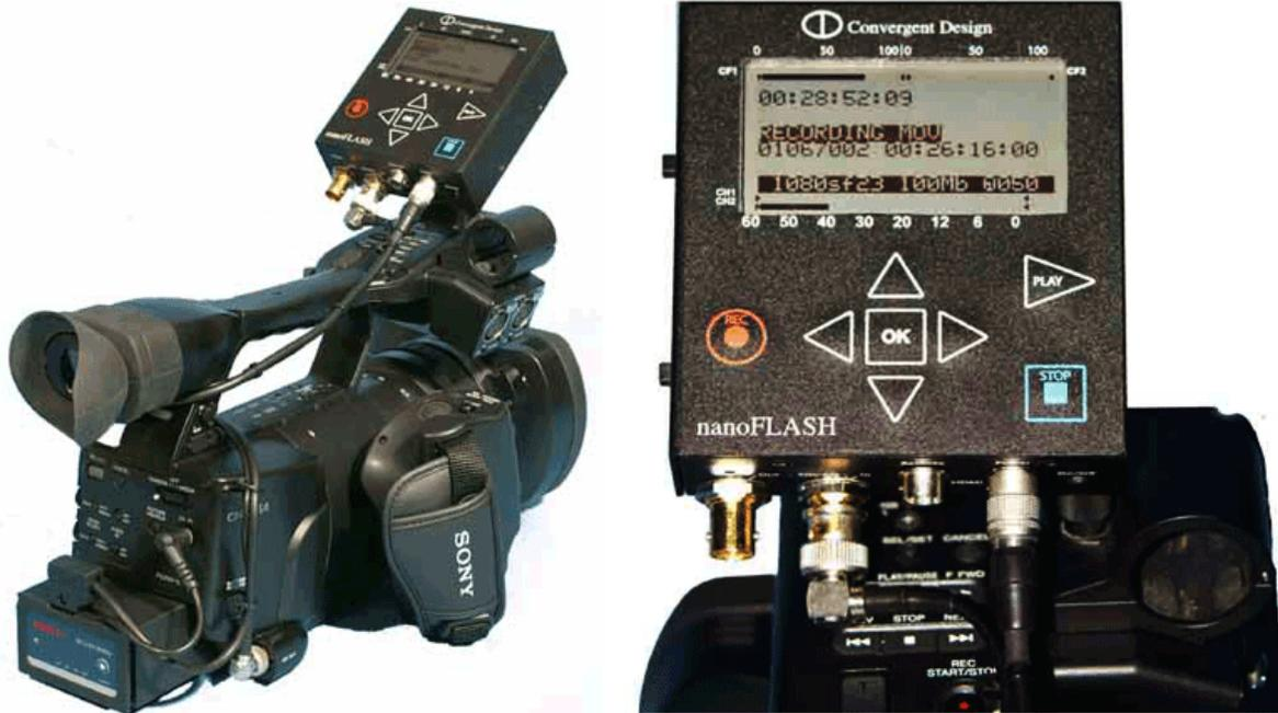
The nanoFlash utilizes two internal processors to record MPEG2 8-bit 4:2:2 video in either Long GOP or iFrame at data rates up to 160Mb/s (Long GOP) or 280 Mb/s (iFrame). Just by comparison, the Sony XDCAM EX cameras output 35Mb/s Long GOP 4:2:0 data and the Sony PDW700 camera outputs 50Mb/s Long GOP with 4:2:2 bit depth.
